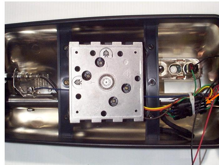
Route the wires as shown, and tie-wrap to the bracket tube.
