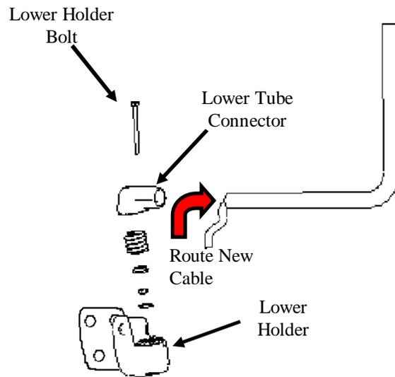
3. Tape the old and new cables together, and route the new cable up the bracket tube, using the existing cable to pull it into location.
