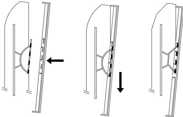
1. Actuate Socket Plate Down, Install Mirror Plate (Align Teeth)
