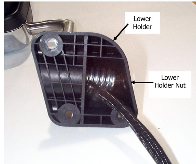
2. Remove the lower holder using a 13 mm socket.
